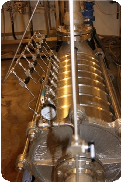
Figure 3. Left: Full-scale Coalescing pump. Right: Example of stepwise sampling of Coalescing pump.
